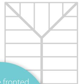
A square fronted duo-pitch roof with a central ridge, providing a flat fronted design that optimises floor space.
